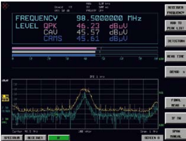
Receiver mode (frequency/level display, bargraph display and continuous realtime IF analysis for set center frequency)
