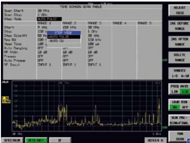
Fast time-domain scan (FFT) with scan table editor
