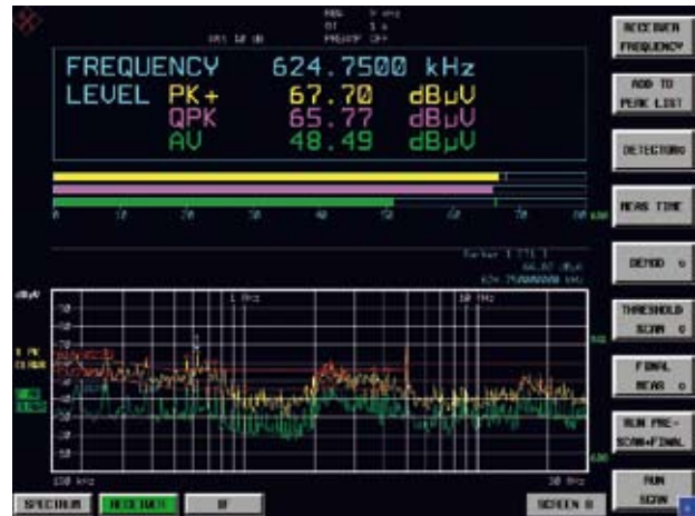
Receiver mode (spectrum display (scan) of preview measurement (PK+AV), limit lines and final measurement results with QP and AV evaluation)
